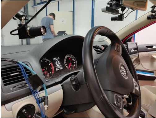
Figure 42 - Mounting of the two ELP machine vision cameras at the windscreen, one facing forward to the traffic, the other facing inwards towards the driver.
