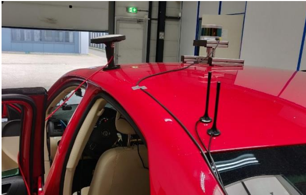
Figure 41 - Mounting of GPS antenna and Velodyne LIDAR on the roof of the TNO vehicle
