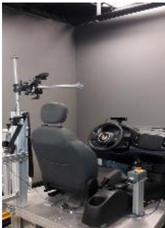
Figure 54 - FOVIO™ eye tracker setup
