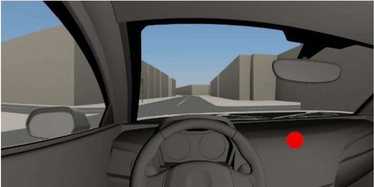
Figure 39 Visualisation of a PET conflict ( PET=0.86s ) from a driver's point of view at the point in time of the highest static hazard level. The size of the red dot represents the static hazard level. This image is taken from a video showing the whole time range of the conflict.
