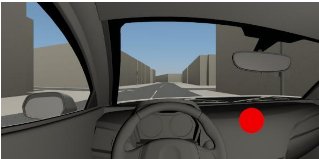
Figure 41 Visualisation of a minimal TTC conflict (minimal TTC = 2.62s ) from a driver's point of view at the point in time of the highest static hazard level. The size of the red dot represents the static hazard level. This image is taken from a video showing the whole time range of the conflict.
