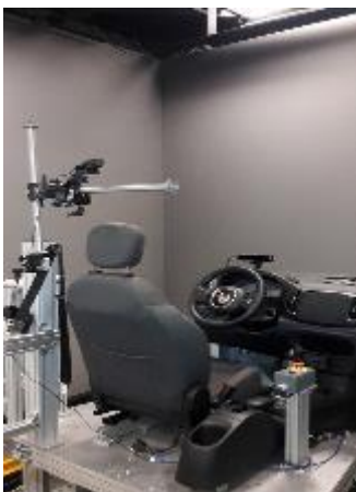
Figure 15 FOVIO eye tracker setup.
