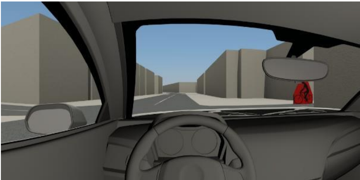
Figure 43 Visualisation of a PET conflict ( PET=0.03s ) from a driver's point of view at the point in time where the cyclist is fully visible for the first time. This image is taken from a video showing the whole time range of the conflict.
